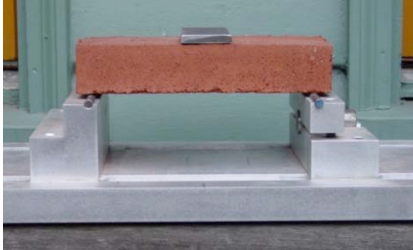
Test fixture with test brick in place
