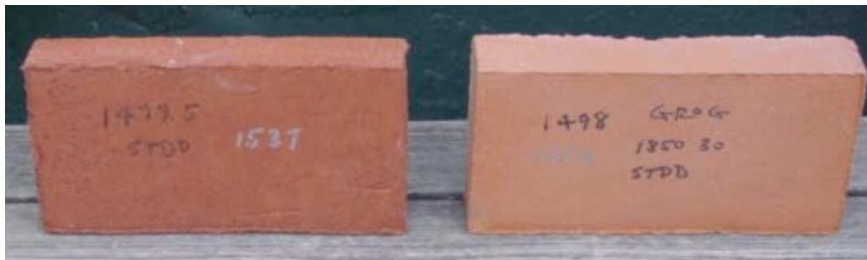
The brick on the left contains 50 percent glass, the brick on the right 50 percent grog. Both were fired to 1850°F.
